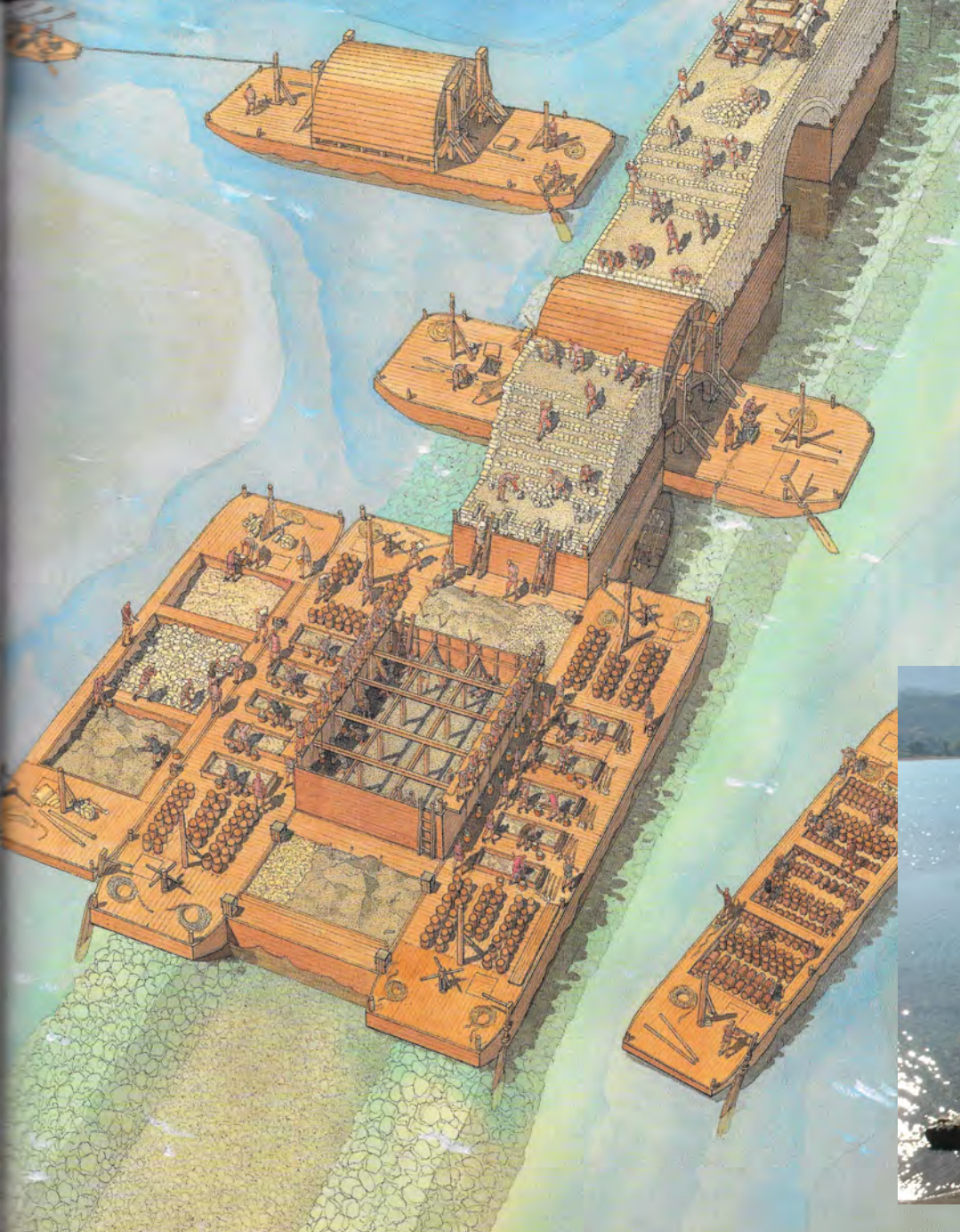
Construction of a breakwater with pilae and arches (Golvin, 2020)
